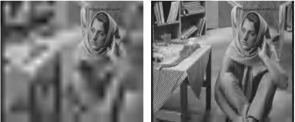
Fig. 3. “Barbara” coded at 0.5bpp using the Maxshift method (left, s = 12 ) and the PSBShift method (right, s = 10 ). The ROI is at the face region and 1/14 of the image size.
